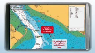
AIS equipment\* displays the icon (pictured above). Precise target survivor information becomes viewable when the chart plotter/ECDIS\* cursor is positioned over the alert icon.
